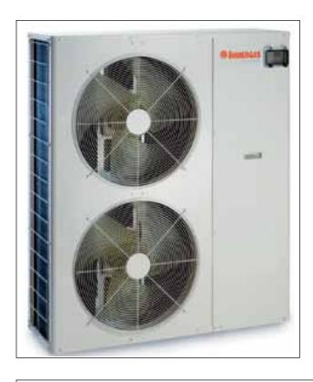
Three-phase reversible air/water Heat Pumps with inverter technology are the Immergas products for air conditioning, named "AUDAX 16 kW" and "AUDAX 18 kW". Designed especially for the production and distribution of heat and cold. They can function independently or coupled with other generators/systems. These machines can also be coupled to a remote storage tank unit for the production of DHW.
